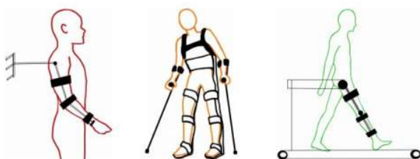
Figure 1-2: Illustration of exoskeleton devices (from left to right): upper limb exoskeleton, lower limb overground exoskeleton, lower limb body weight supported exoskeleton. Source: [3]
